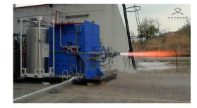
Skyroot announced the triumphant 200-second fireendurance test of enhanced, fully 3D-printed 'Dhawan-II' Cryogenic engine that will power the upper stage of Vikram-2
