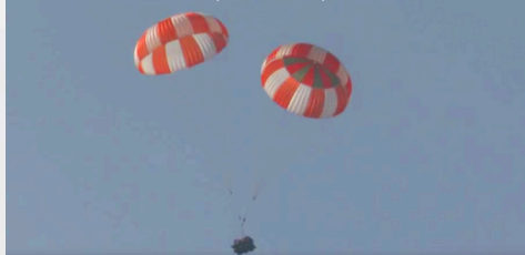
GAGANYAAN PARACHUTE DECELERATION SYSTEM Integrated Main Parachute Airdrop Test (IMAT -03)
