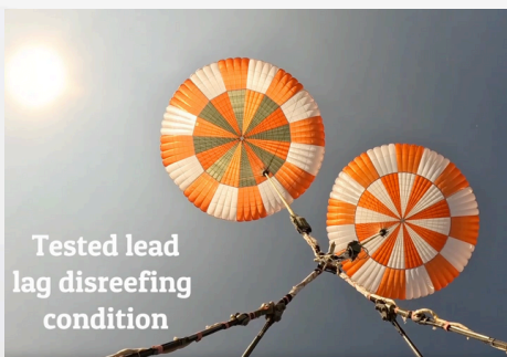
GAGANYAAN PARACHUTE DECELERATION SYSTEM Integrated Main Parachute Airdrop Test (IMAT -03)
